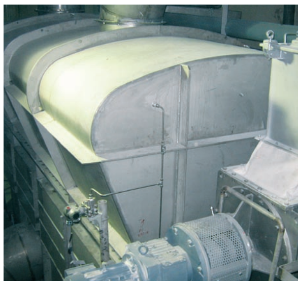
Fluidized-bed cooler with feed lock
